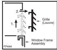
**Fig. 12** Louvre installation and removal.
